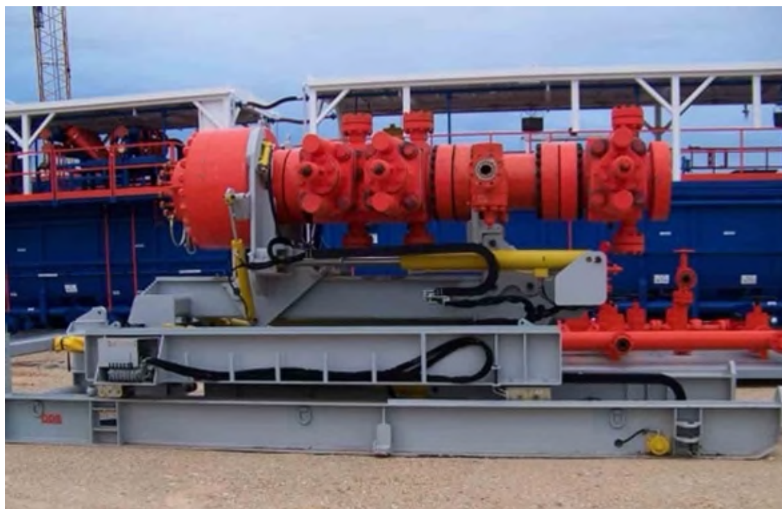
Figure 4. BOP handling system
