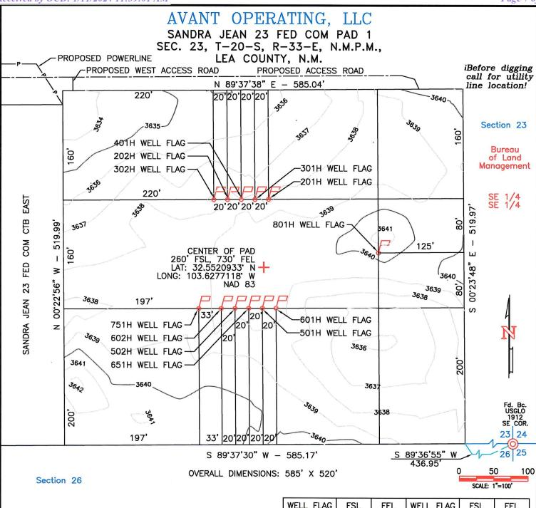
1. ALL BEARINGS, DISTANCES & COORDINATES SHOWN ARE BASED UPON THE NEW MEXICO STATE PLANE COORDINATE SYSTEM, EAST ZONE, NAD 83, IN U.S. SURVEY FEET.
