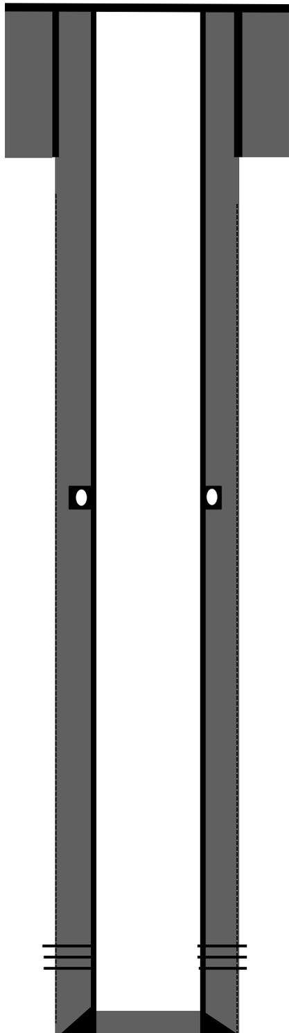
8-5/8" J-55 24# casing @ 320'. Cemented with 265 Cu.ft Class B.
