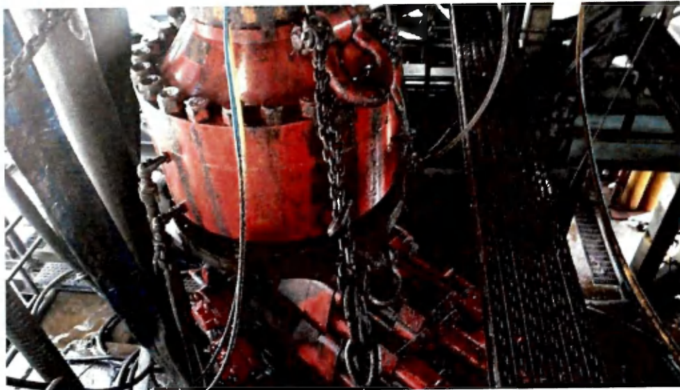
Figure 1: Winch System attached to BOP Stack
