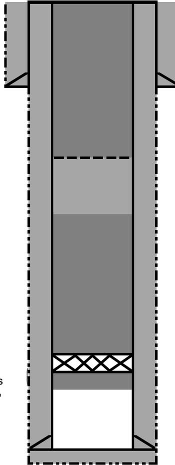
12-5-2023: Cut off WH. TOC at 28' in 5 1/2" casing and at 14' in 8 5/8" casing. Install P&A marker, top off casings and cellar with poly pipe and 28 sx.
