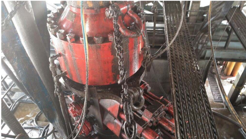
Figure 1: Winch System attached to BOP Stack
