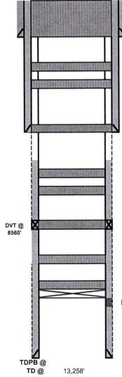
13 3/8 35 & 48# CSG @ 428 10. Perf'd @ 500'. Sqz'd 180 sx class C cmt @ 500' & circulated to surface.
