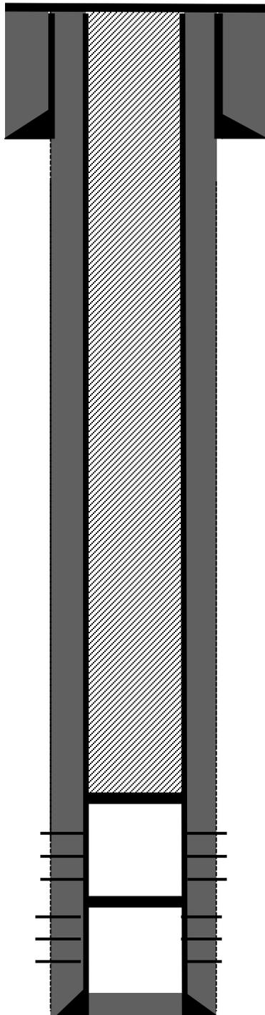
7", 20# casing @ 122'. Cemented with 70 sks Class B cement w/2% CaCl2 .
