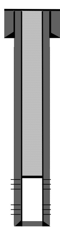
7" 20# casing @ 120'. Cemented with 50 sks, 59 Cu.ft Class B cement. Hole size: 8-3/4". Circulate 2 bbls cement to surface.
