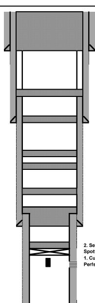
9.Perf'd @ 700'. Established injection rate in 9 5/8 only. Pressured up on 13 3/8. ND BOP, & Spool. Sqz'd 260 sx class C cmt @ 700' & circulated to surface in only 9 5/8. Tagged plug @ 20'. Spotted 5 sx class C cmt @ 20' to surface.
