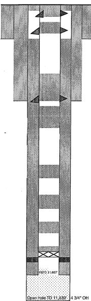
SURFACE EQUIPMENT SURFACE ANCHORS: Last Test Date: 50 sxs 500-surface 50 sxs 1330-857 CBL showed Cement from CIBP to 1990' 50 sxs 4230-3825 50 sxs 5600' 25 sxs 7100' 25 sxs 7940' 25 sxs 8900° CIBP 11500' Pressure tested
