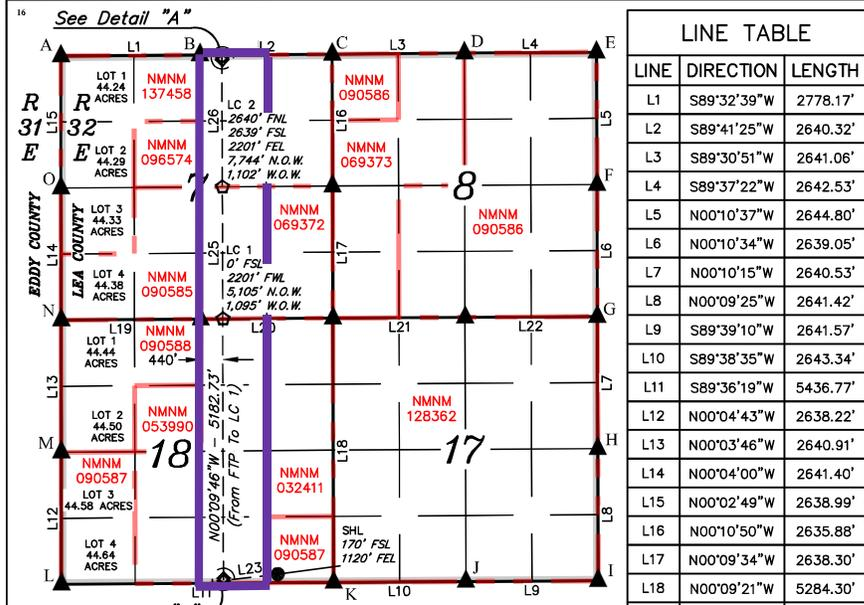
LINE TABLE with columns: LINE, DIRECTION, LENGTH. Lists 27 lines (L1-L27) with bearings and lengths.
