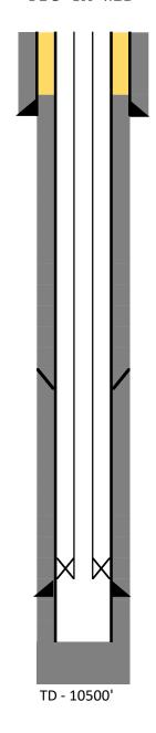
17-1/2" hole @ 926' 13-3/8" 54.5# csg @ 926' w/780 sx-TOC-Surf-Circ
