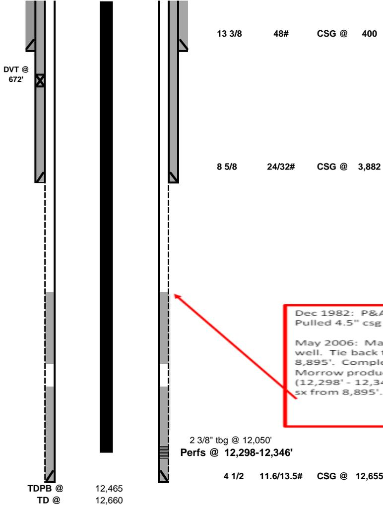
Dec 1982: P&A original well. Pulled 4.5" csg from 8,895'.
