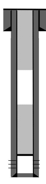
8-5/8" 24# casing @ 128'. Cemented with 100 sks, 118 Cu.ft Class B cement. Hole size: 12-1/4". Circulate 4 bbls cement to surface.
