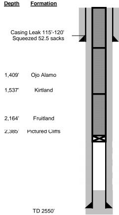
**Plug #3: 7" Surface casing shoe:** Mix and pump 25 sx Class G cement plug from 746' to 5' and circulate good cement out casing.
