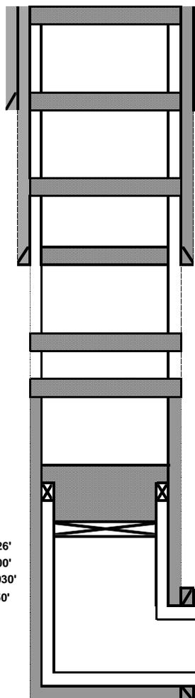
**Plug #9:** Perf'd @ 100'. ND BOP. Sqz'd 70 sx class C cmt @ 100' & circulated to surface in 9 5/8". Topped off well with 35 sx class C cmt
