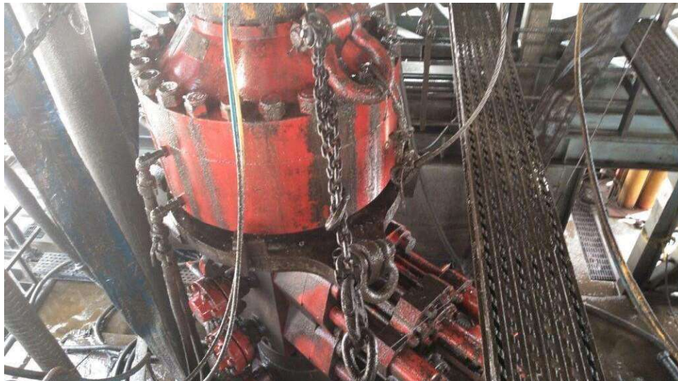
Figure 1: Winch System attached to BOP Stack
