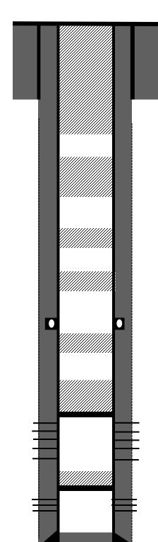
8-5/8" J-55 24# casing @ 354'. Cemented with 250 sks, Type 5 cement w/ 3% CaCl2. Circulated 18 bbls cement to surface. Hole size: 12-1/4
