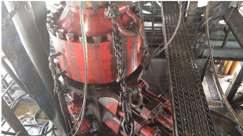
Figure 1: Winch System attached to BOP Stack
