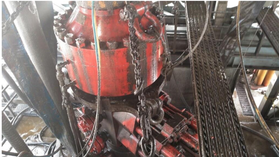
Figure 1: Winch System attached to BOP Stack
