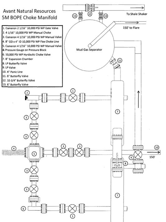
Choke Manifold Diagram
