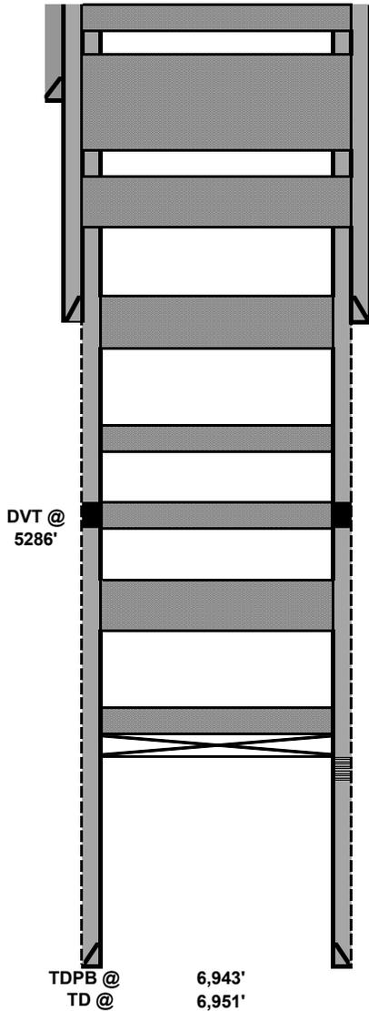
**Plug #8:** Perf'd @ 100'. Sqz'd 30 sxs class C cmt @ 100' & circulated to surface.
