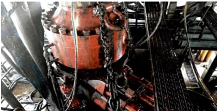
Figure 1: Winch System attached to BOP Stack
