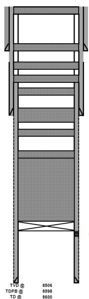
Plug #9: Perf'd @ 100'. Sqz'd 73 sxs class C cmt @ 100' & circulated to surface.
