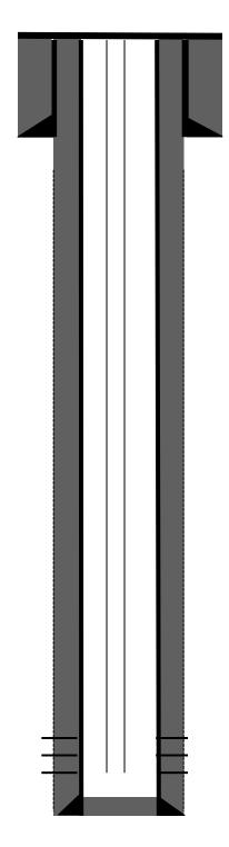
7" 20# casing @ 126' Hole size 9-7/8" Cemented w/ 50 sks Class B neat 2% CaCl2 w  $\frac{1}{4}$ #/sk celloflake (59 cu ft). Circ 2 bbls cement to surface
