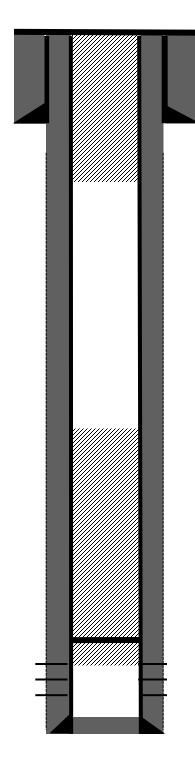
7" 20# casing @ 126' Hole size 9-7/8" Cemented w/ 50 sks Class B neat 2% CaCl2 w ¼#/sk celloflake (59 cu ft). Circ 2 bbls cement to surface
