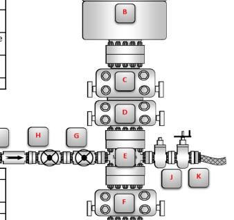
**Choke line Pressure Part** Size Description Rating 3" 5,000 HCR (gate valve) K 3" 5,000 Manual HCR (gate valve) Wellhead **Pressure Part** Size Description Rating 13-5/8" 5,000 FMC 5M/10M wellhead
