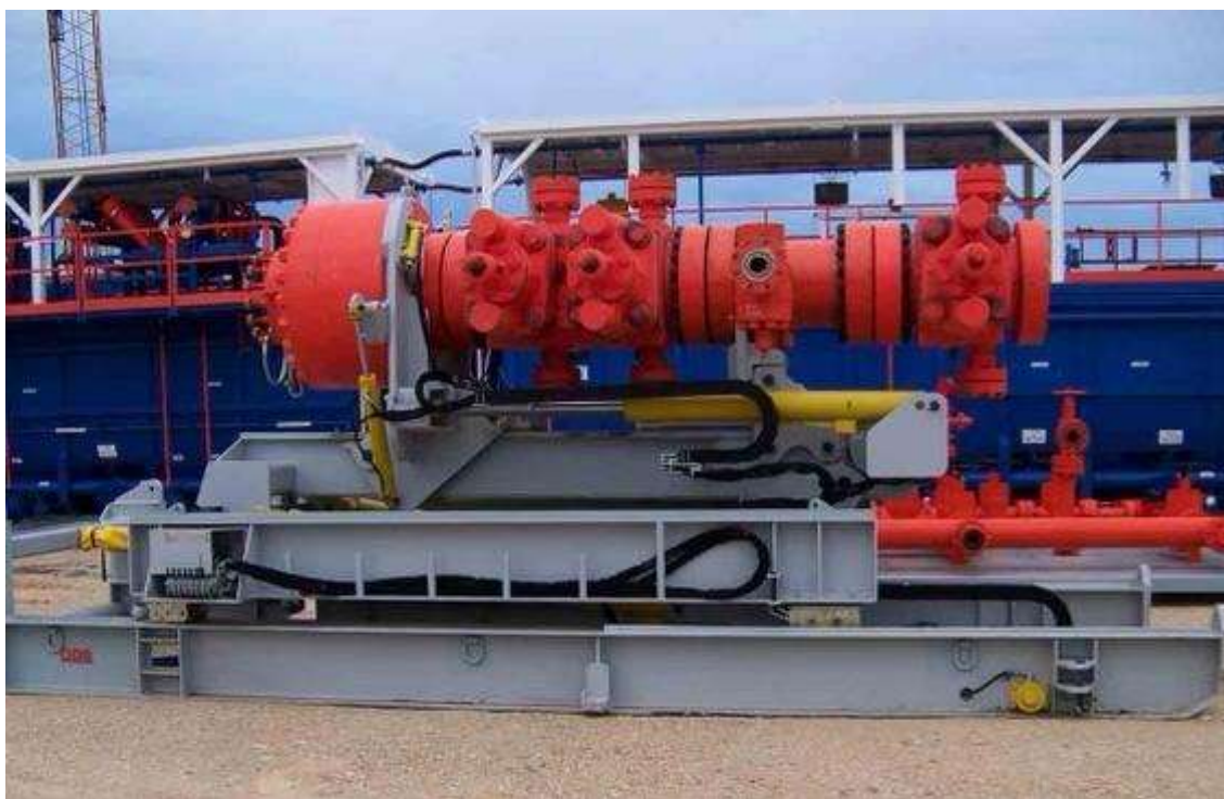
Figure 4. BOP handling system
