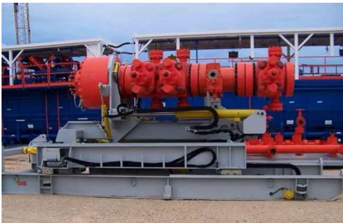
Figure 4. BOP handling system
