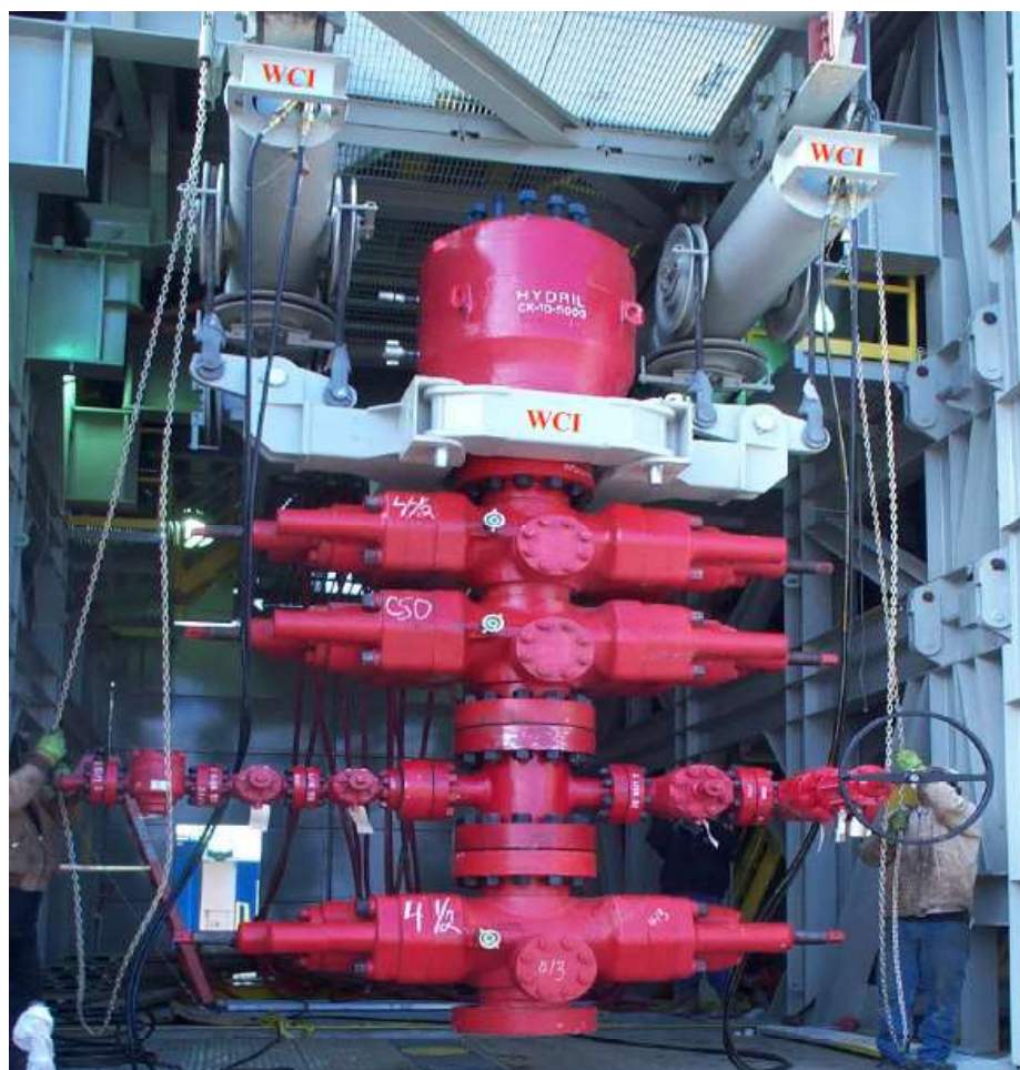
Figure 3. BOP handling system
