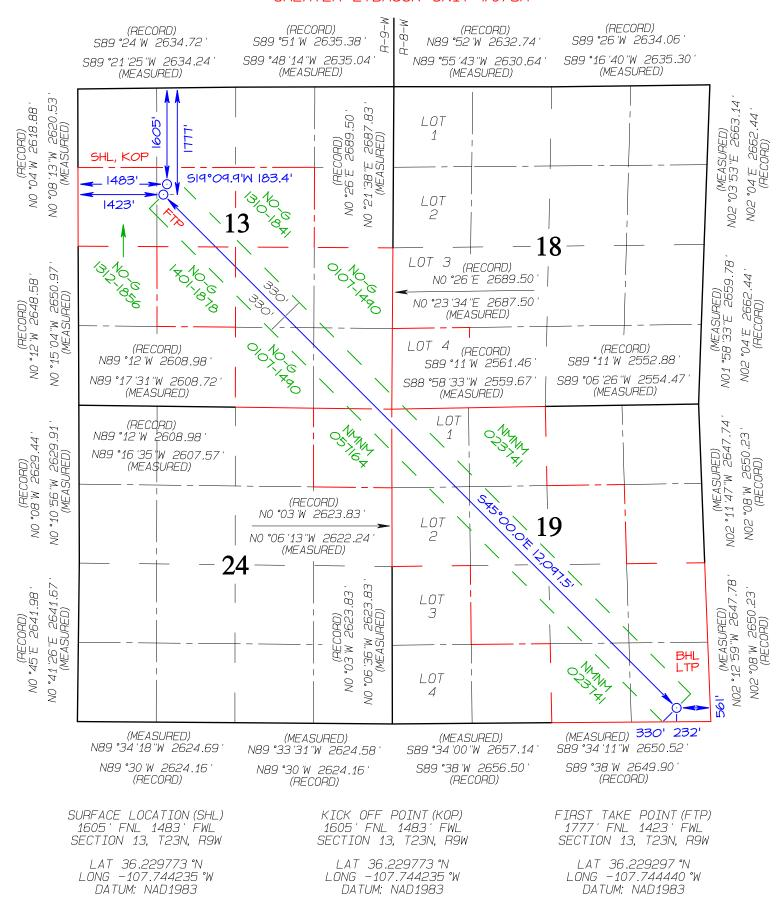
BOTTOM HOLE LOCATION (BHL) 232' FSL 561' FEL SECTION 19, T23N, R8W
