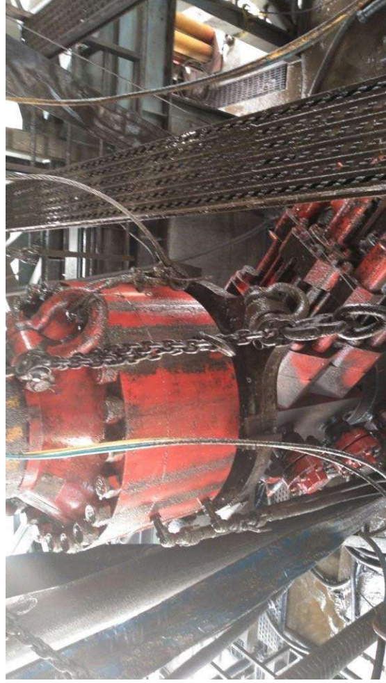
Figure 1: Winch System attached to BOP Stack
