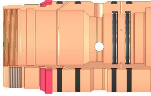
Annular packoff with both external and internal seals
