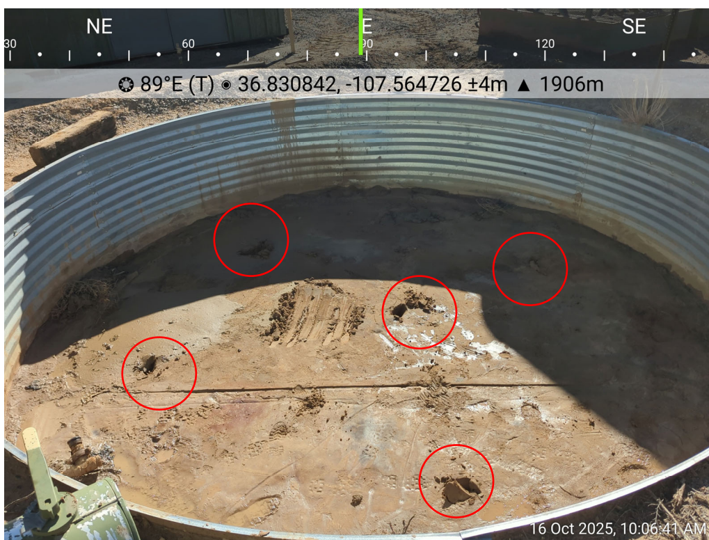
Photo 4: Five-point composite sample (SS45) collected below base of BGT.
