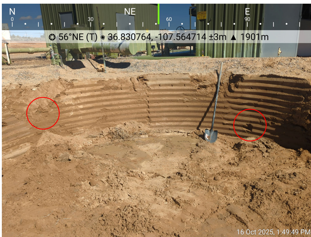
Photo 6: Five-point composite sample (SS47) collected from sidewalls of BGT location, view east.
