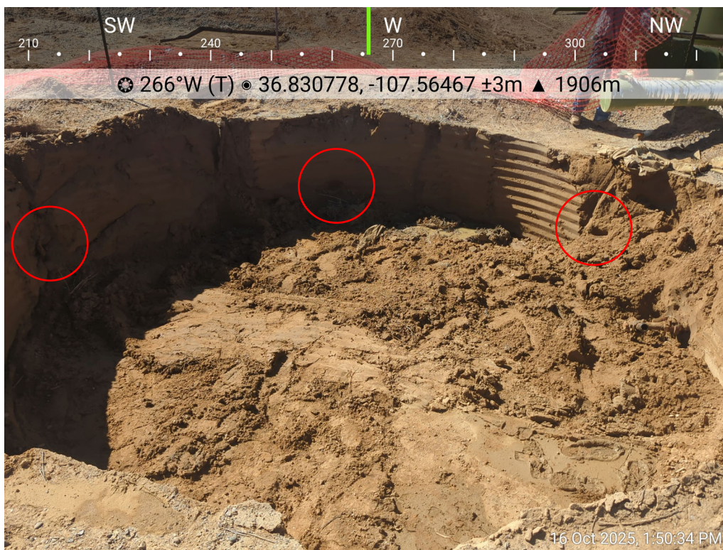
Photo 5: Five-point composite sample (SS47) collected from sidewalls of BGT location, view west.
