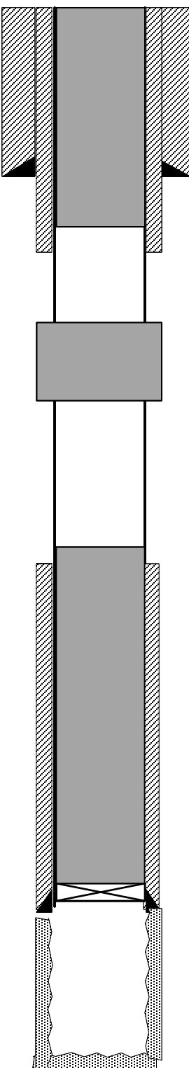
Plug 3 (Surf Shoe) – Perf 188' – attempt to circulate – established injection rate 3 bpm @ 700 psi – BLM ok with 25 sx attempt – pump/ squeeze 25 sx, pressuring up, WOC Tag 121' – pump to surface 17 sx cmt – top off, cut and weld below ground monument ok with BLM Top off with 66 sx cmt Plug 188-surf
