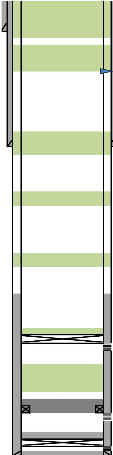
Plug #7: (Surf Shoe/Surface) Circulate 114 sxs (49in/65out) class C cmt from 450' to 0'. Verify and Bubble test.
