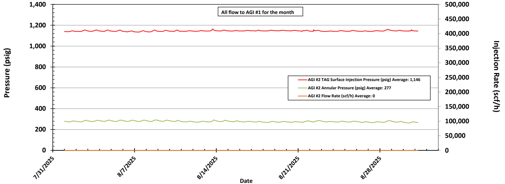
Figure #5: Linam AGI #2 Injection Pressure, Rate and Casing Annulus Pressure
