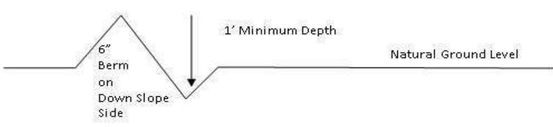
All lead-off ditches shall be graded to drain water with a 1 percent minimum to 3 percent maximum ditch slope. The spacing interval are variable for lead-off ditches and shall be determined according to the formula for spacing intervals of lead-off ditches, but may be amended depending upon existing soil types and centerline road slope (in %);
