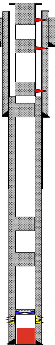
Perf &amp; circulate w/60sx Class C (250-0) Verify at surface- Cap Shoe
