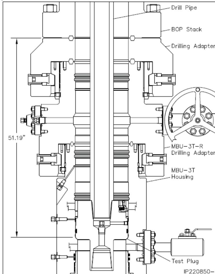
Figure 5. Cactus 5M wellhead with BOP quick connect
