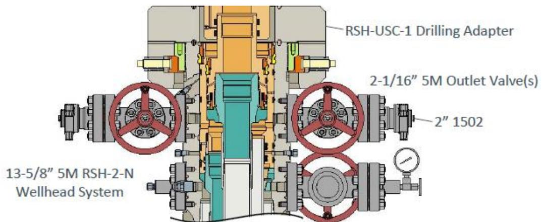
Figure 6. Vault 5M wellhead with BOP quick connect
