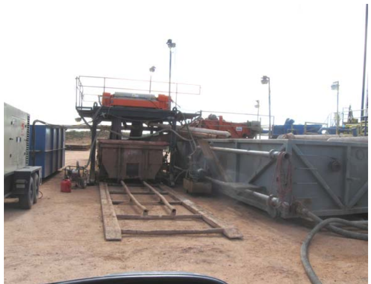
Above: Centrifugal Closed Loop System
