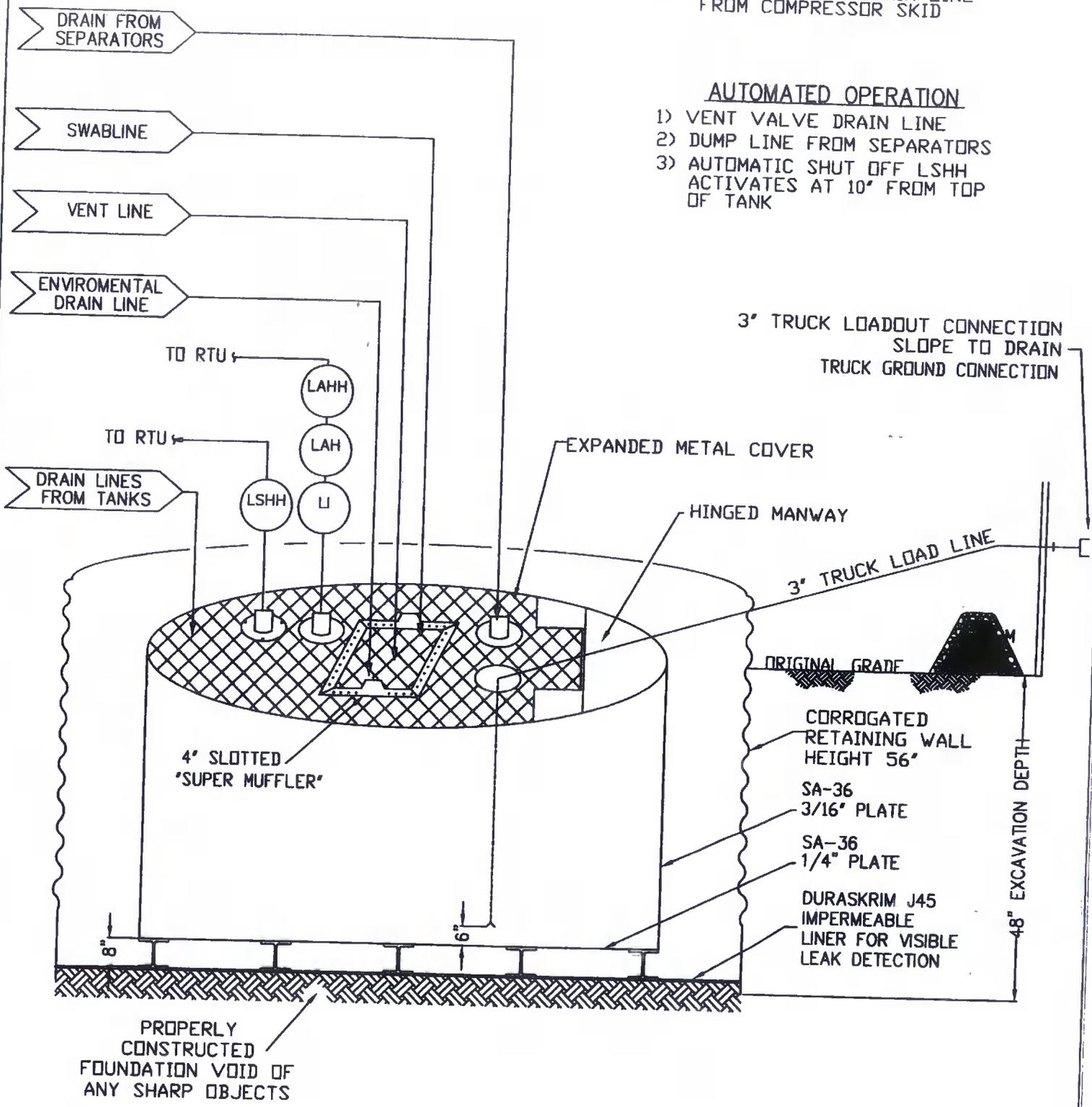
3" TRUCK LOADOUT CONNECTION
