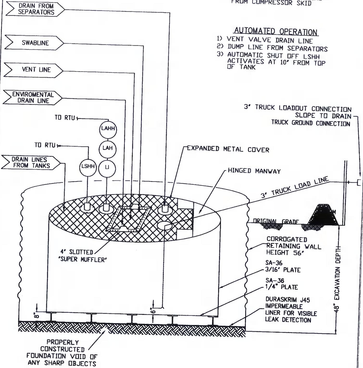
3" TRUCK LOADOUT CONNECTION
