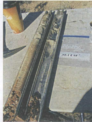
Photograph 11. Split spoon sample; top of Chinle Formation at 27'.
