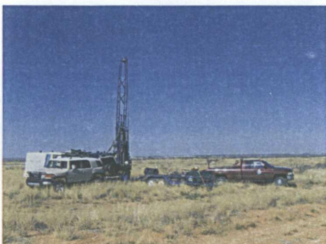
Photograph 1. Rodgers set up on MP-1 with CME-75 combination HSA and air rotary drill rig and related equipment.
