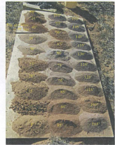
Photograph 16. Cuttings samples at 5-foot intervals below ground surface (as shown) at MP-3 (top of Chinle Formation as indicated).
