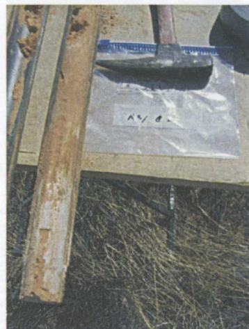
Photograph 3. Split spoon sample; top of Chinle Formation at 27'.
