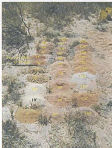
Photograph 13. Cuttings samples at 5-foot intervals below ground surface (as shown) at MP-2 (top of Chinle Formation as indicated).
