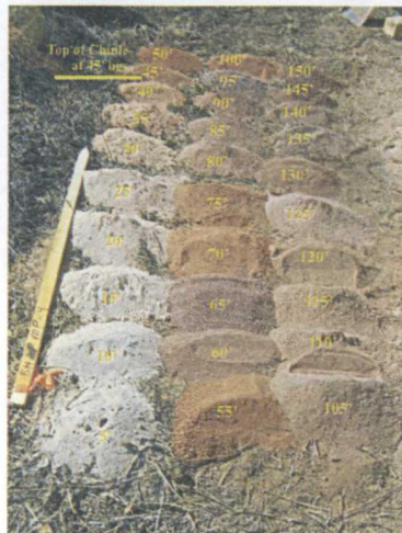
Photograph 18. Cuttings samples at 5-foot intervals below ground surface (as shown) at MP-4 (top of Chinle Formation as indicated).
