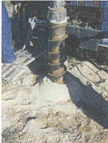
Photograph 10. HSA drilling caliche in boring MP-2.
