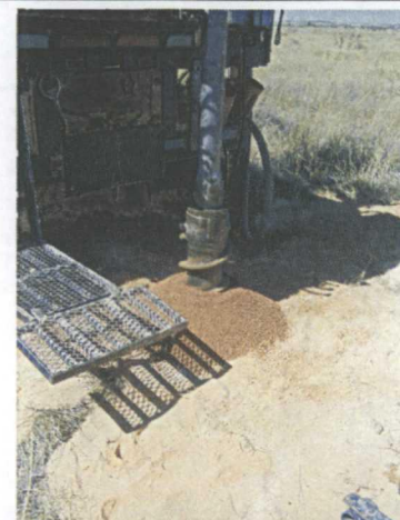
Photograph 4. HSA drilling top of Chinle Formation at MP-1.
