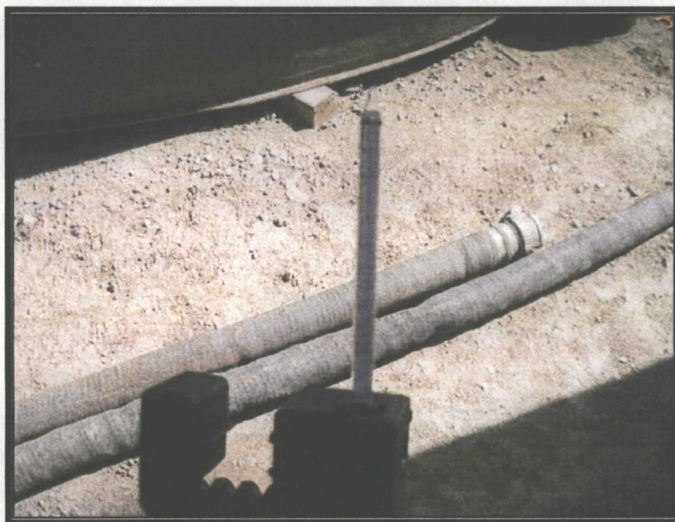
Photo 6: "Dräger" Tube used for H 2 S Monitoring (View 3)
