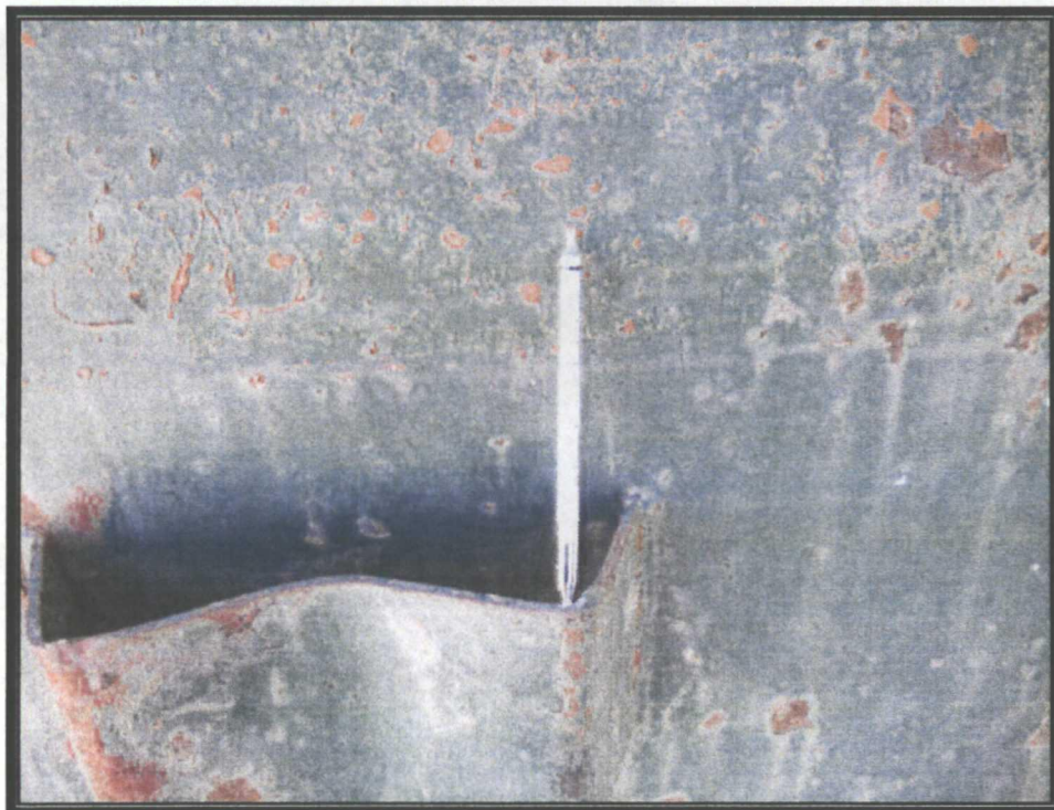
Photo 7: "Dräger" Tube used for H 2 S Monitoring (View 5)
