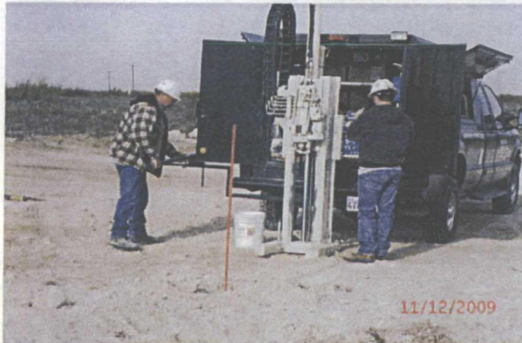
drilling SB #1 at 15 ft east of the former junction
