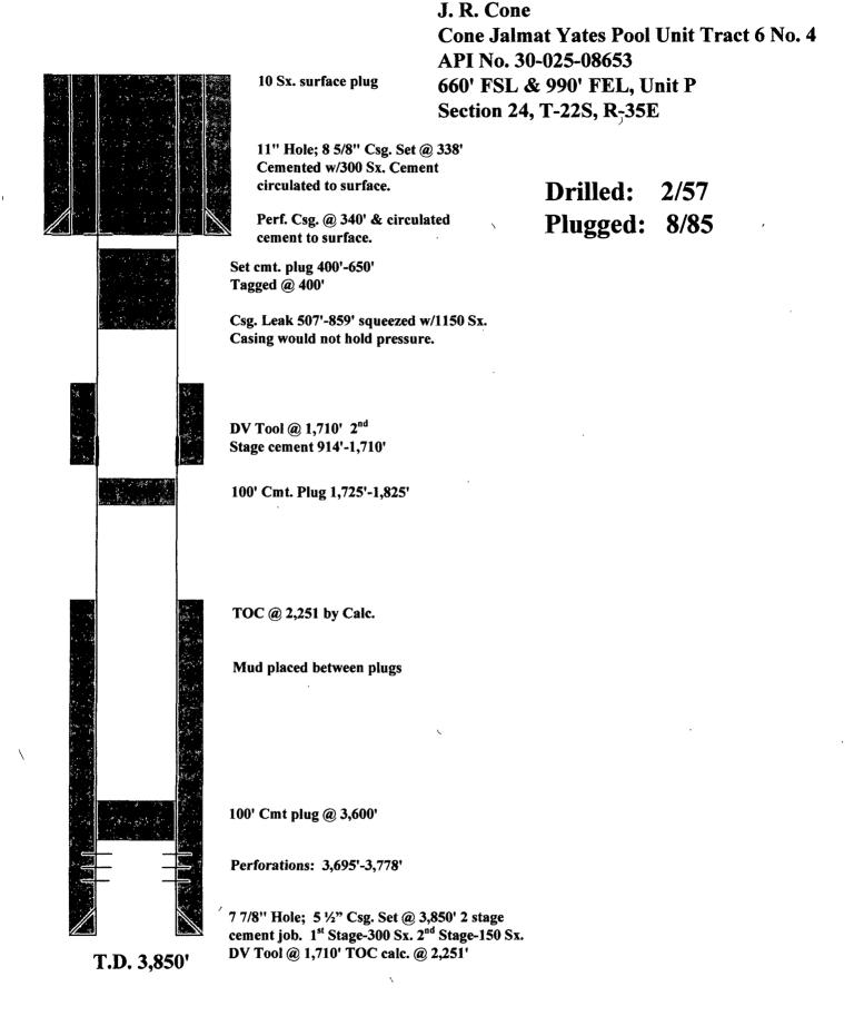
Form C-108, CJYPU 401 & 605 Quantum Resources Mgt., LLC PA Schematic CJYPU Tract 6 No. 4
