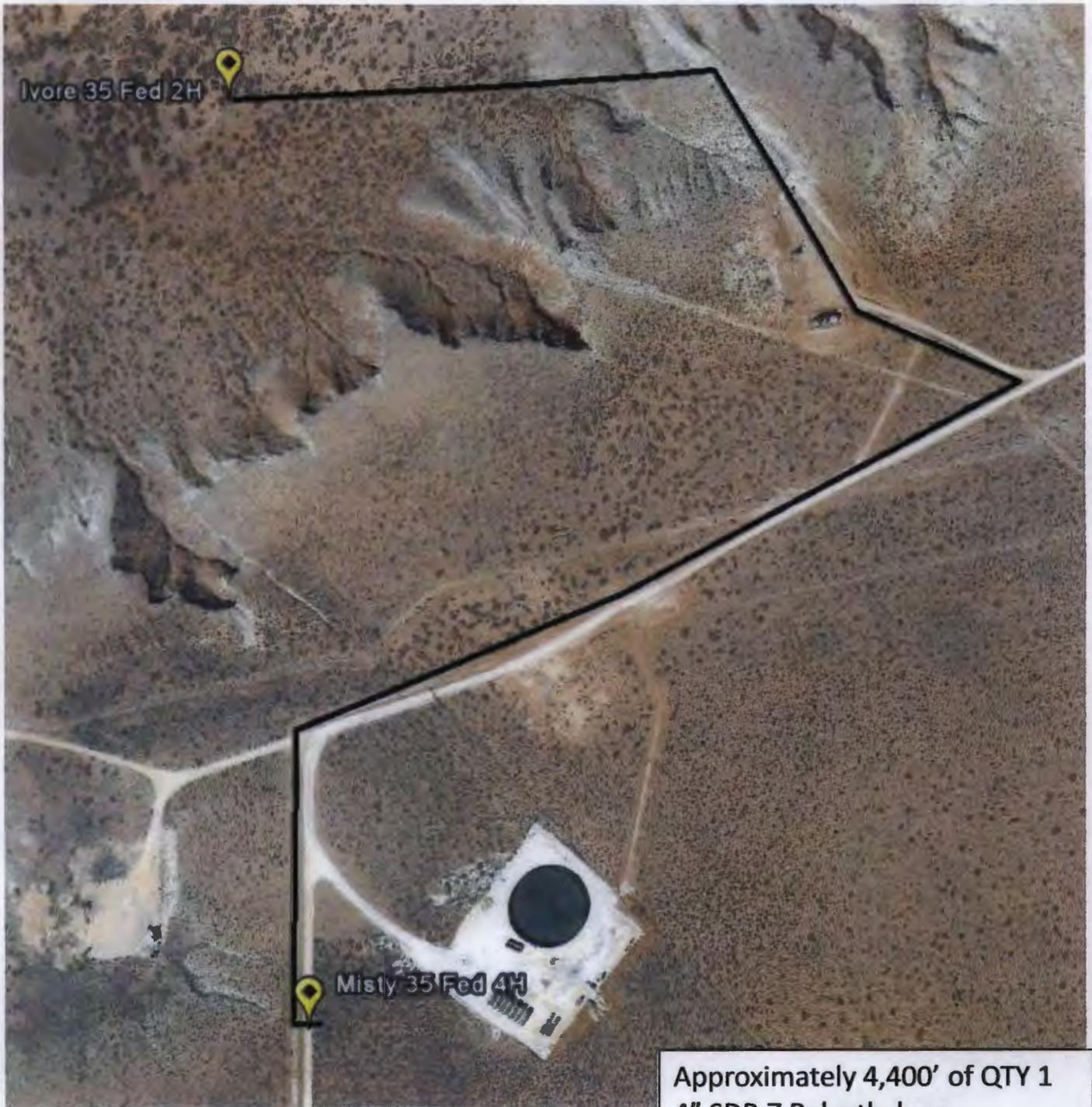
Approximately 4,400' of QTY 1 4" SDR 7 Polyethylene production flowlines (oil, gas, and produced water) to be laid on the surface Misty 35 Fed 4H Battery Location. Operating Pressure < 125 psig
