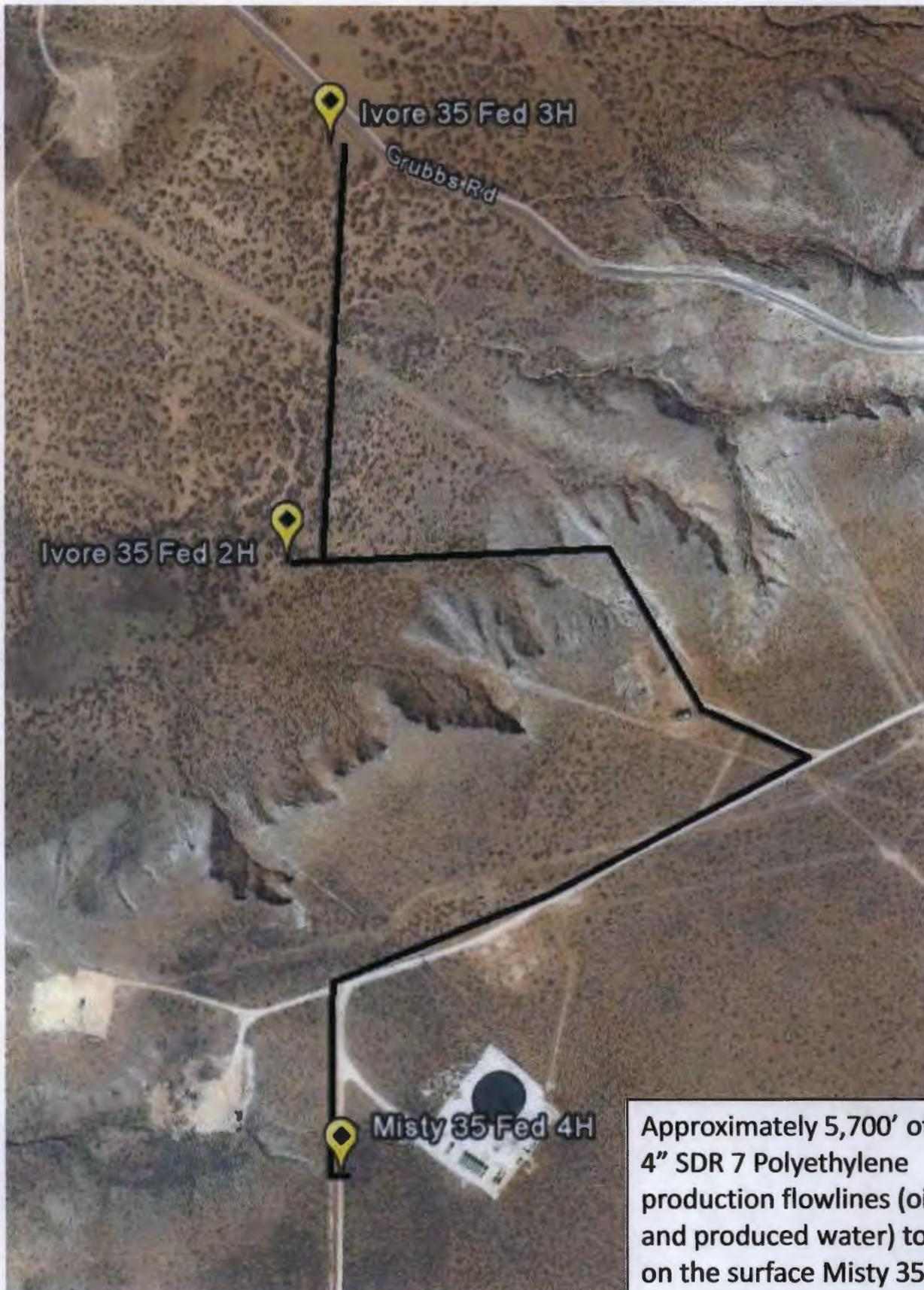
Approximately 5,700' of QTY 1 4" SDR 7 Polyethylene production flowlines (oil, gas, and produced water) to be laid on the surface Misty 35 Fed 4H Battery. Operating Pressure < 125 psig
