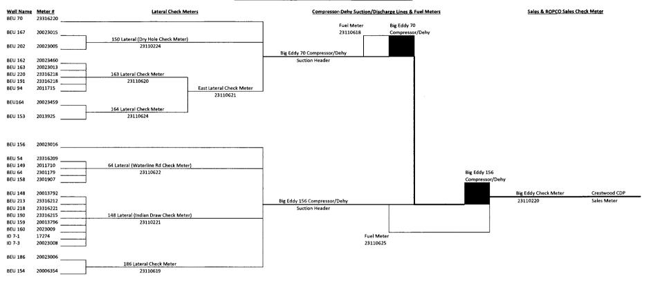
Production from these wells goes through production units located at each well site. The condensate and water are separated and stored in tanks at each site and trucked off location. The gas is metered at each battery location before being transported to the Big Eddy 156 Compressor/Dehydrator
