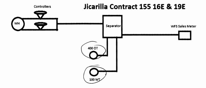
Testing Procedure: For testing/allocation purposes, the DK will be shut off via the controller for 24 hrs once a month to test the MV production.
