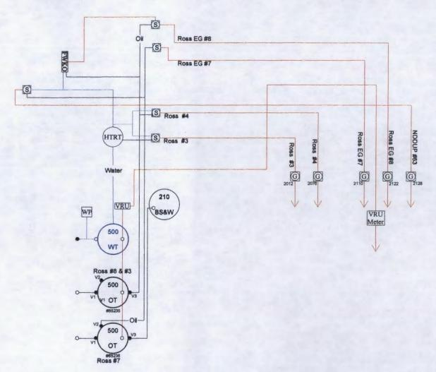
Sales: From Tank Gauge to Truck Tank Tank Valve Position for sales Tank #65235 (Ross EG #8) or #65236 (Ross EG #7)
